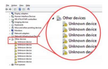
Figure above: Unknown devices in Device Manager
